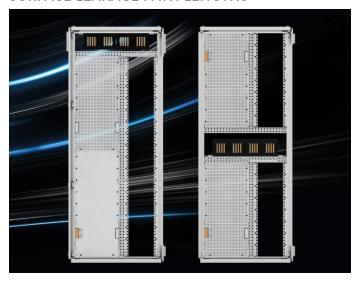
Rated impulse-withstand voltage and rated insulation voltage are taken into account in specifying the insulation gaps and surface leakage path lengths between different circuits. On the busbar systems ensuring easy mounting, thanks to the modular structure, it is designed to make insulation gaps between phase-phase and phase-neutral 70mm in the smallest point. Since the assembly locations on the support rails are already designated, possibilities of mistake during production are eliminated.
