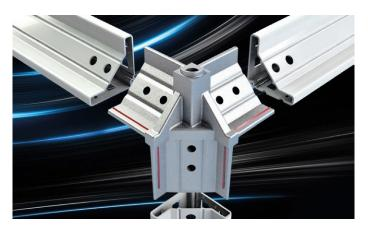
• Grounding hooks located on aluminium corner combination that joins main carcass structure are mounted to the internal surface of the unpainted profile tightly and abrasively. Thus the grounding continuity is ensured in all profiles and the parts that will be mounted to them.
