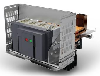
• Open type circuit breaker sections are separated from top and bottom sections and input-output terminals inside its own section with sheet metal, and input-output terminals are separated from each other with plastic insulation sheet. This way, accidental contact of operator with conductors is prevented / limited. (In Form 2a-4b options)
